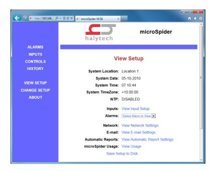
This page allows inspection of all microSpider's configurable parameters, without making any changes.
