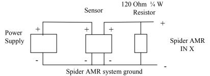
(ii) Voltage inputs may require up to two external resistors:
