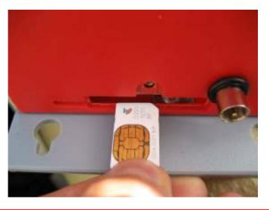
IMPORTANT: You should feel slight resistance while pushing the card into the slot. If you do not or you can freely move the SIM from side to side by more than 1 mm you have missed the slot. You must remove the SIM and try again!
