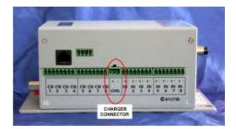
Every Spider AMR incorporates a battery management system supporting 12V sealed lead acid batteries with capacities up to 10 Ah.
