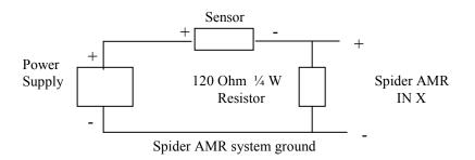
(ii) **4-WIRE 0 - 20 mA and 4 – 20 mA** current loop sensors require an external 120 Ohm,  $\frac{1}{4}$  W resistor:
